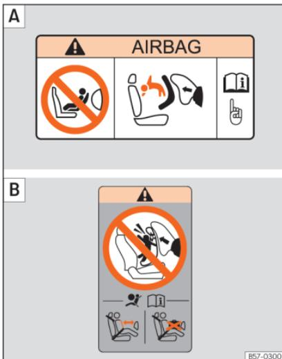
**Fig. 37** Airbag adhesives - version 2: on the passenger-side sun blind **A** and on the rear frame of the front passenger's door **B**.
