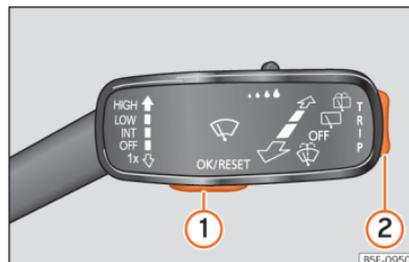
**Fig. 136** Windscreen wipers lever: control buttons.
