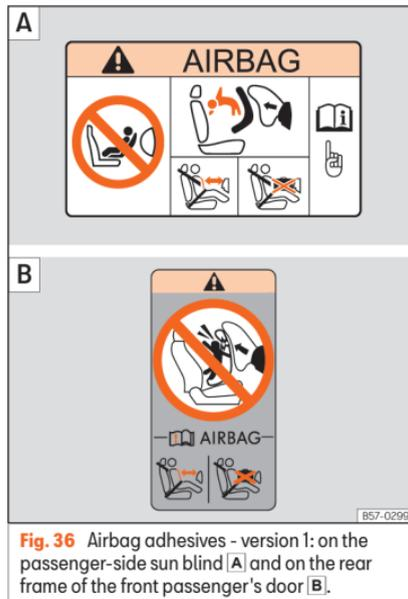
**Fig. 36** Airbag adhesives - version 1: on the passenger-side sun blind **A** and on the rear frame of the front passenger's door **B**.
