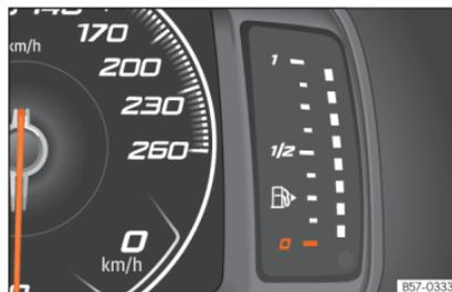
**Fig. 132** Digital instrument panel: fuel gauge.
