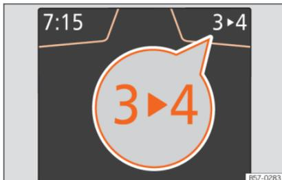
**Fig. 261** Instrument panel: gear-change indicator (manual gearbox).
