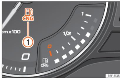
**Fig. 133** Analogue instrument panel: natural gas gauge
