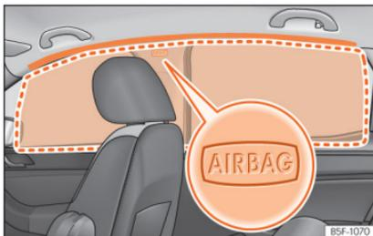
**Fig. 34** Location of head-protection airbags.
