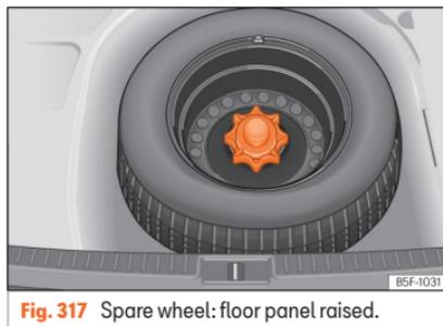
**Fig. 317** Spare wheel: floor panel raised.
