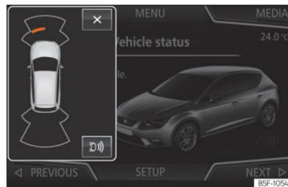
**Fig. 286** Miniature indication of automatic activation.
