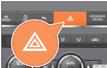
**Fig. 46** Dashboard: switch for hazard warning lights.
