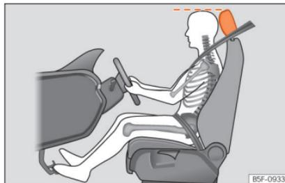
**Fig. 88** Correct head restraint position for the driver.
