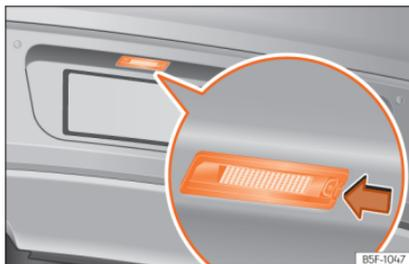
**Fig. 121** In the rear bumper: number plate light.
