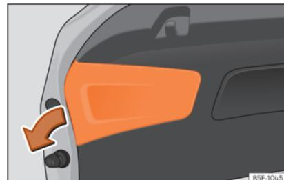
**Fig. 119** Remove the cover from the rear lid
