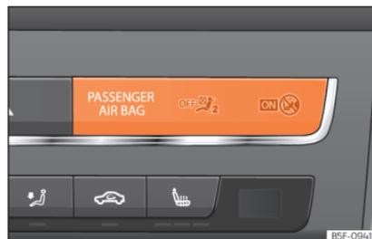
**Fig. 99** Dashboard: control lamp for deactivated front passenger airbag in centre console.
