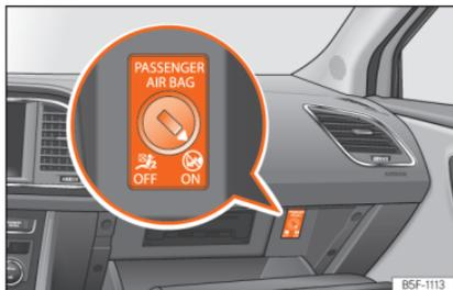
**Fig. 28** Front passenger front airbag switch.
