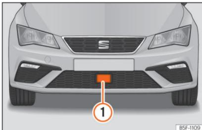
**Fig. 271** On the front bumper: radar sensor.
