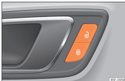
**Fig. 5** Driver door: central locking switch.
