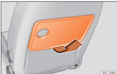
**Fig. 166** Left-hand front seat: folding table.
