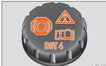
**Fig. 65** Engine compartment: brake fluid reservoir cap.
